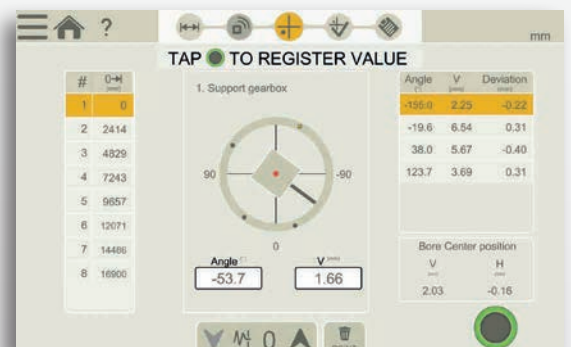
Bore center program, measuring view, first position. Measure 3–50 points at each position (Multipoint). Individual points can be remeasured at any stage.
