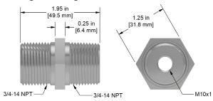
DM915-1A 316L Stainless Steel, ½-14 NPT to ¾-14 NPSM Mounting Bushing with M10x1 Threaded Hole
