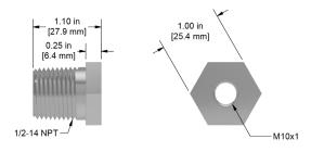
DM914-1A \_\_\_\_\_\_ 316L Stainless Steel, %-14 NPT to %-14 NPT Mounting Bushing with M10x1 Threaded Hole
