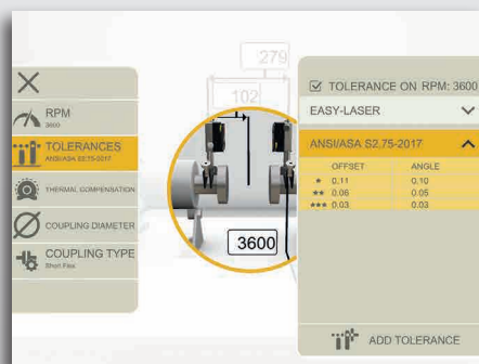
Tolerance check (pre-set or custom)
