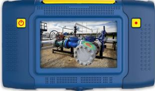
SonaVu<sup>™</sup> is a multi-frequency acoustic imaging camera that blends visual and auditory senses to bring fugitive emissions, natural gas, and oil leaks into focus. One problem facing refineries and oil and gas (O&G) plants is how to identify and eliminate sources of leakage into the atmosphere.
